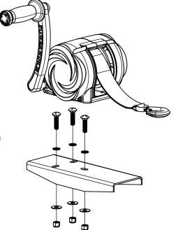
The winch should be mounted with ¾ mounting hardware to meet SAE Standard J1853 for boat trailer winches.
