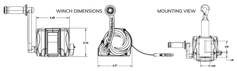
The Powerwinch Premier Series 2000 Trailer Winch is made with precision gears, plated for maximum corrosion resistance. The winch has a gear ratio of 4.75:1 to ensure easy, smooth operation, and includes a 12-tooth ratchet gear for high-resolution cranking.
