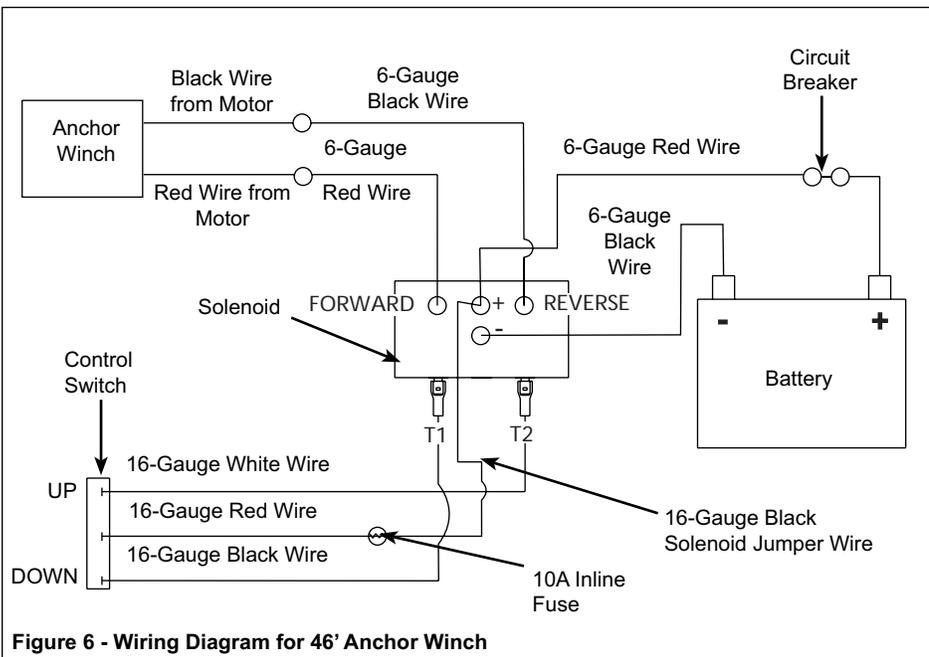
Figure 6 - Wiring Diagram for 46' Anchor Winch
