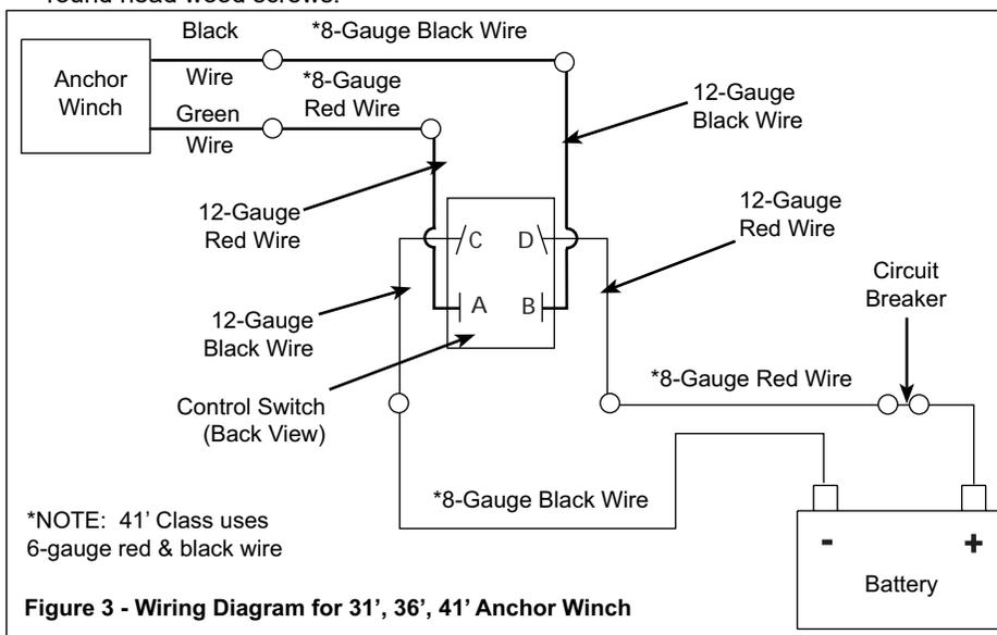
Figure 3 - Wiring Diagram for 31', 36', 41' Anchor Winch
