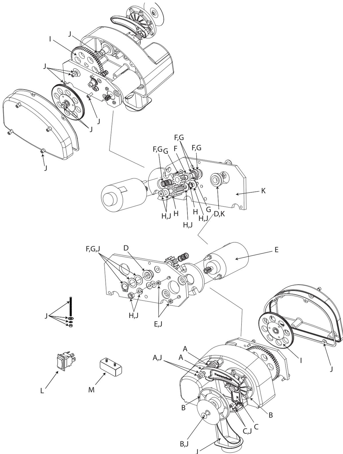
Figure 7 - Replacement Parts Illustration for 31', 36', 41' Class Anchor Winch
