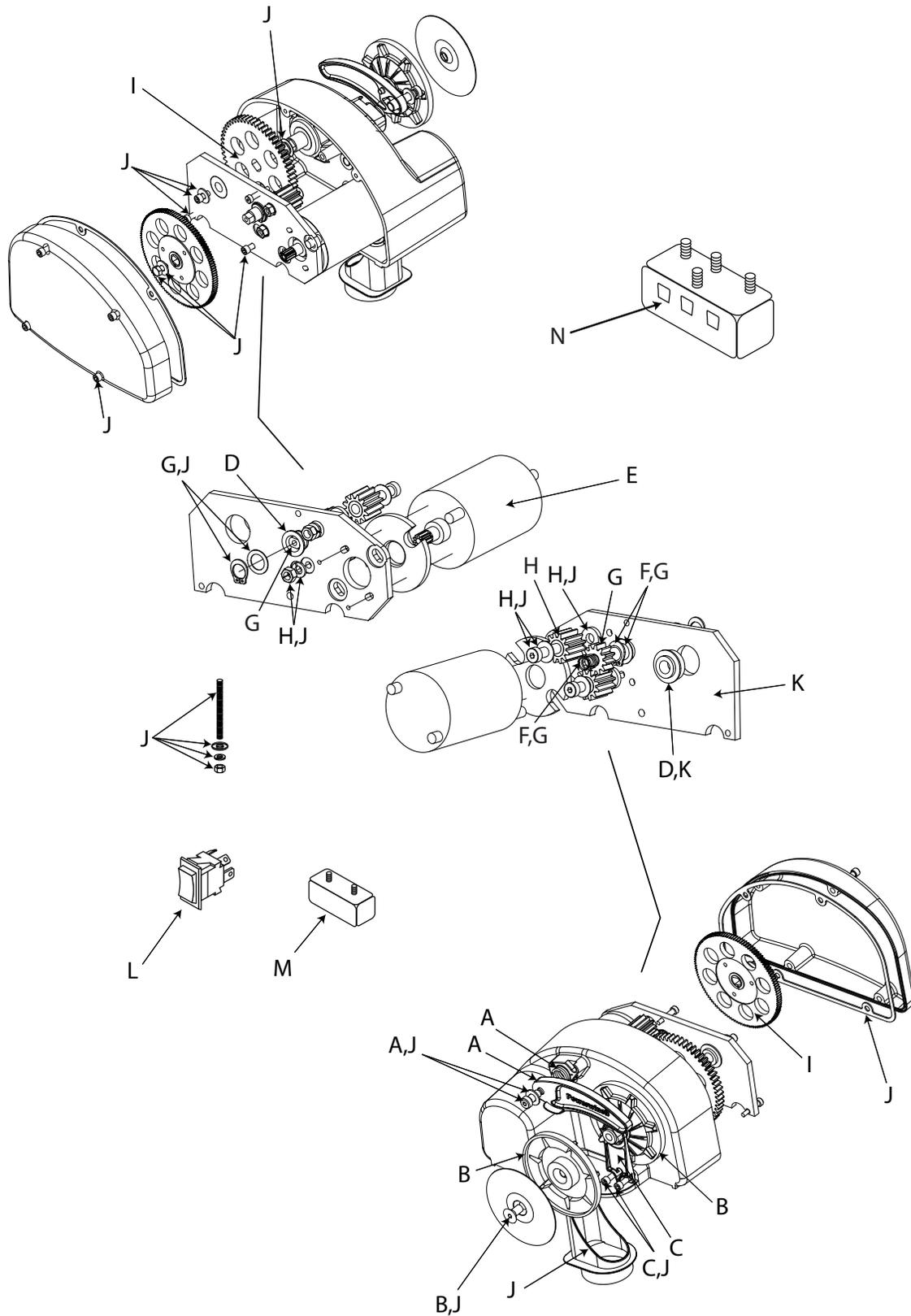
Figure 8 - Replacement Parts Illustration for 46' Class Anchor Winch
