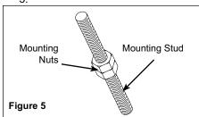
5. Gently guide winch over rode glide so loop on anchor winch housing slides over deck insert. Slide three mounting studs into three mounting holes in deck. Feed wiring harness from underside of winch through 5/8" hole.
