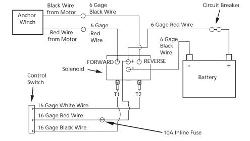
Figure 6 - Wiring Diagram for 45' Anchor Winch
