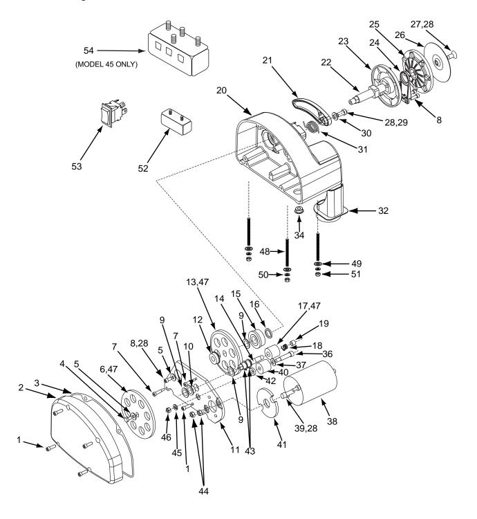
Figure 7 - Replacement Parts Illustration for 30', 35', 40', 45' Class Anchor Winch
