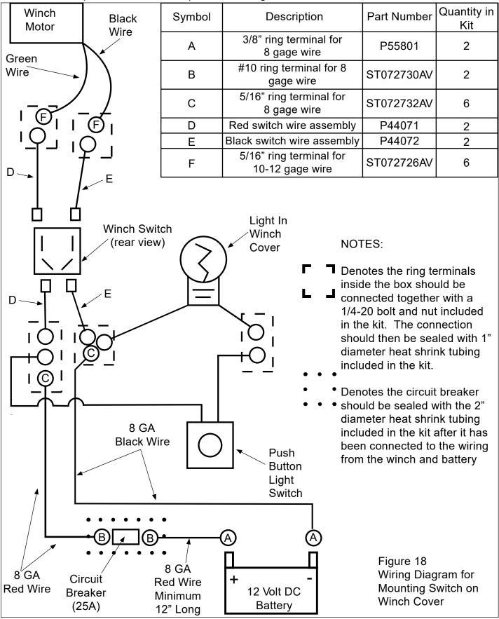
**Step 5.** Assembling Winch Cover and Unit Test
