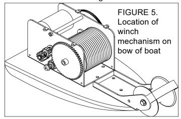
Make sure the centerline of the rope spool is in line with the center line of the bow roller as shown in Figure 6. If the winch is not properly aligned with the bow roller, the winch will not operate properly.
