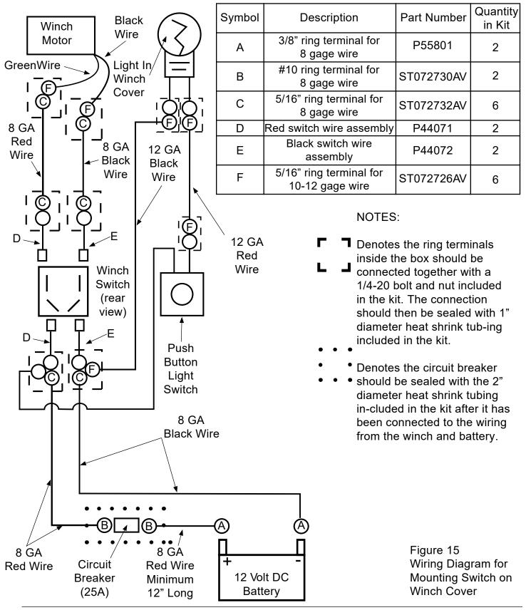
**Step 4** Installing the switch and wiring the winch to the battery. (continued).
