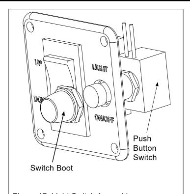
Figure 17. Light Switch Assembly. Insert push button switch through hole in switch plate and secure with switch boot.
