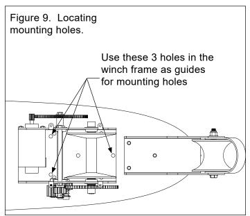
After marking the holes as shown, remove the winch and drill the holes through the deck using a 1/4" drill bit.
