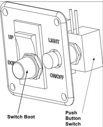
Figure 13. Light Switch Assembly.
