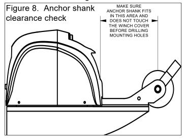
Once it is certain the anchor will not hit the cover of the winch, remove the cover. Using a permanent marker, mark the deck through the mounting holes in the winch frame. Figure 9 shows which holes in the winch frame should be used as mounting holes.
