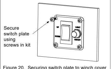
Figure 20. Securing switch plate to winch cover
