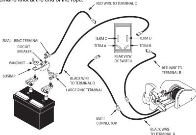
Figure 2. Deckmate 19 Wiring
