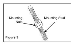
so loop on anchor winch housing slides over deck insert. Slide three mounting studs into three mounting holes in deck. Feed wiring harness from underside of winch through 5/8" hole.
